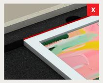
The red line indicates that the frame is lower than the top of the foam. This way there's space for the artwork to move during transit and will cause damage.
